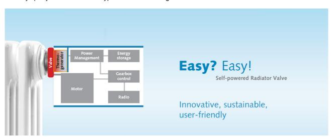
If, in exceptional cases, the storage voltage drop below a certain limit, the actuator reports this status to the room controller and takes the protection position (50% valve opening or maintains the set value, whichever is the higher). Subsequently, the actuator goes to sleep and waits until the memory is re-charged by the thermoelectric generator back to a sufficient level. As soon as enough energy is available, the actuator resumes normal operation.
